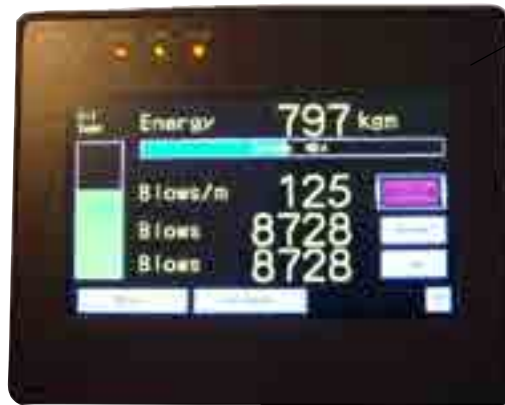
INTERFACE SCREEN MOUNTED ON POWER PACK
