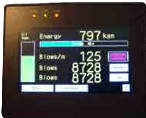
INTERFACE SCREEN MOUNTED ON POWER PACK
